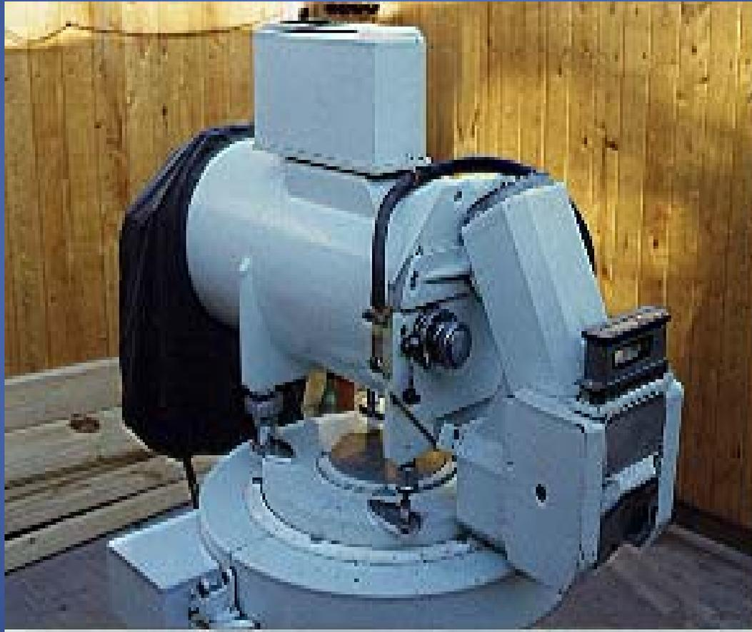
*Automated Photoelectric Astrolabe Telescope PAII (1992 -2007)*
