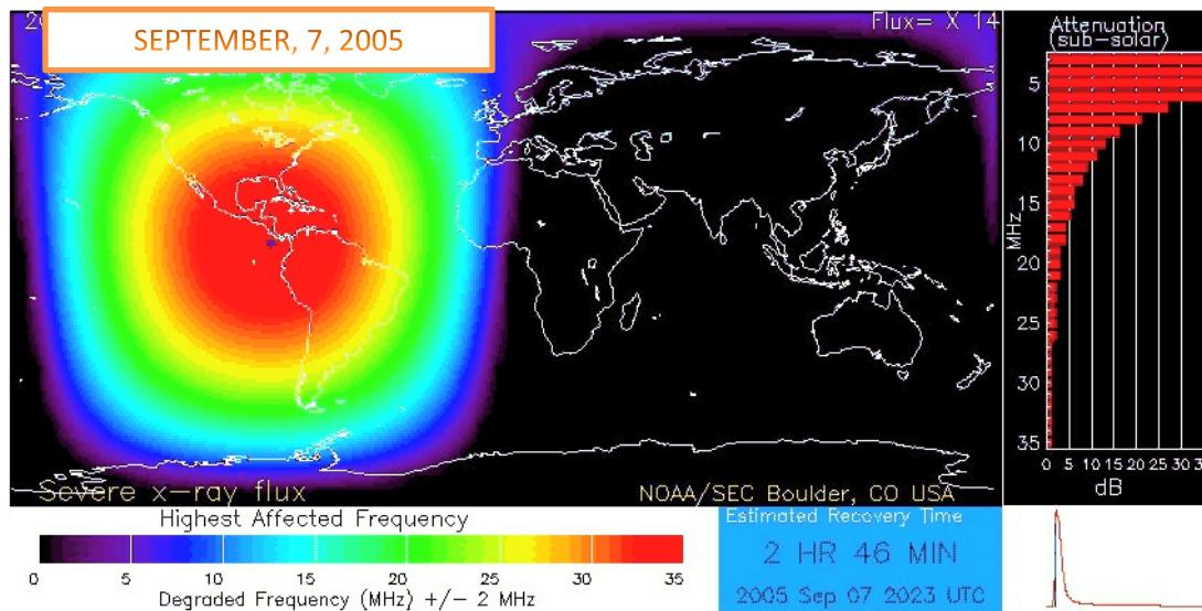
$$\text{HAF [MHz]} = 10 \cdot \log[\text{flux\_1\_8 (W/m}^2\text{)}] + 65$$
